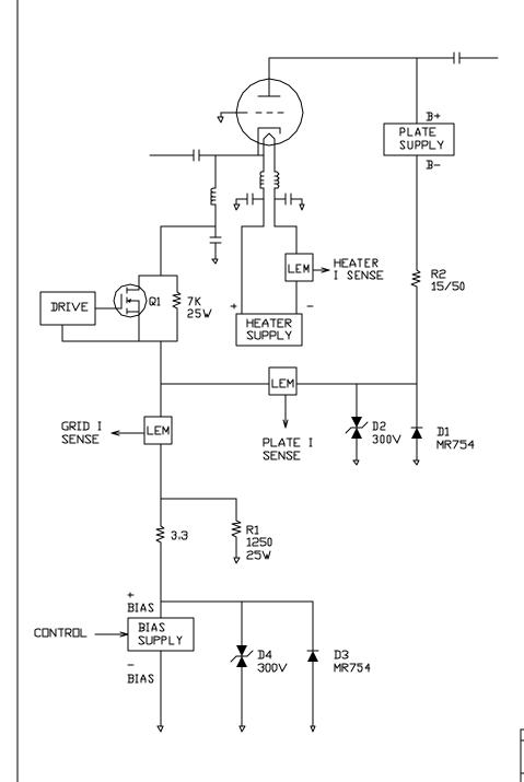
R2 LIMITS CURRENT FROM PLATE SUPPLY IN EVENT OF TUBE ARC OR OTHER PLATE CIRCUIT FAULT.
